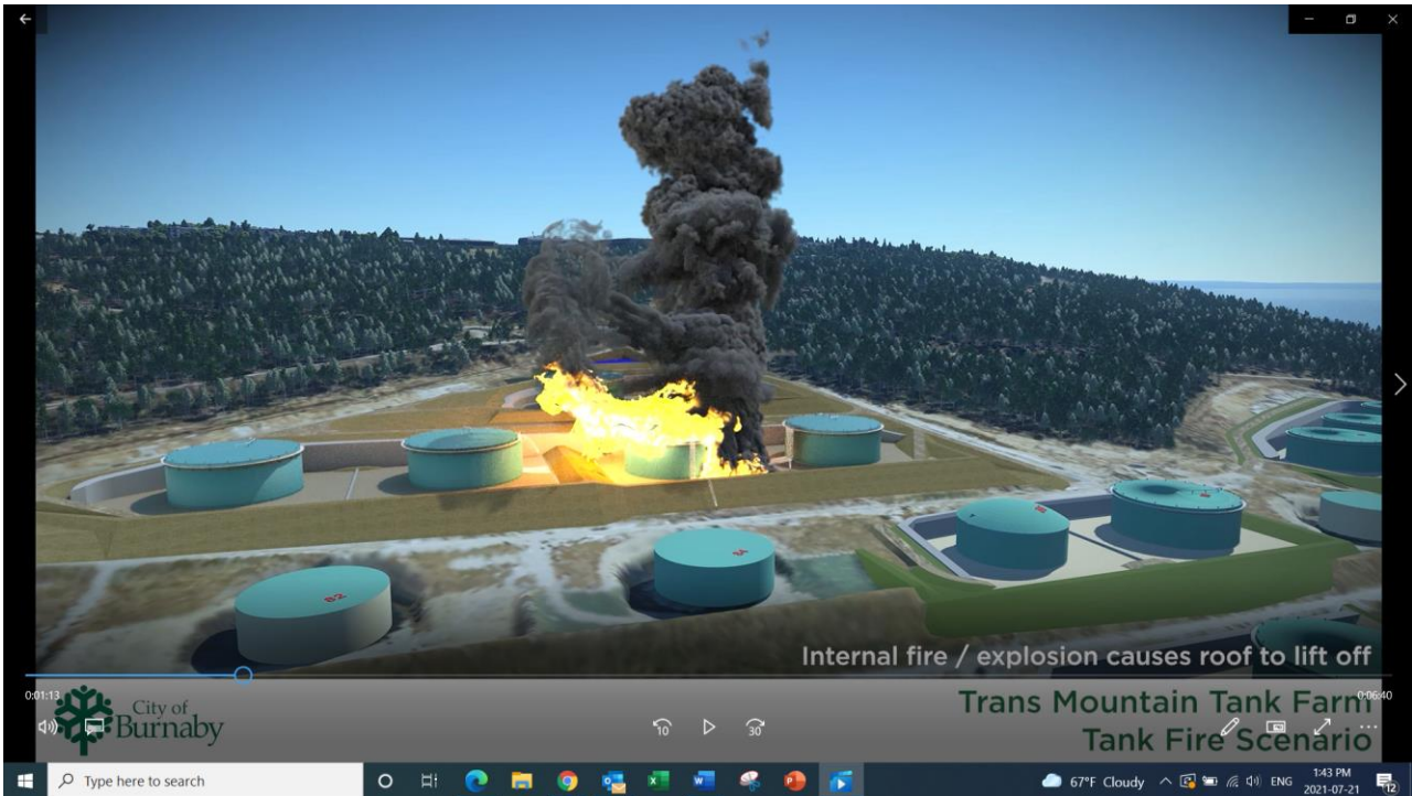
Above: An internal fire / explosion can cause the roof to lift off.
