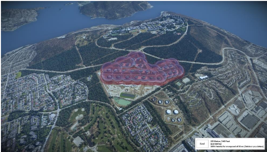
Burnaby Tank Farm and full surface fire heat map- Red Zone.
