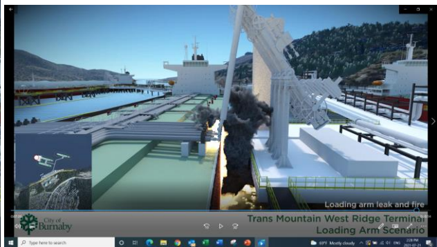
View #4- View from a position between the berth and tanker. Dynamic model on right shows oil leak onto water with fire.
