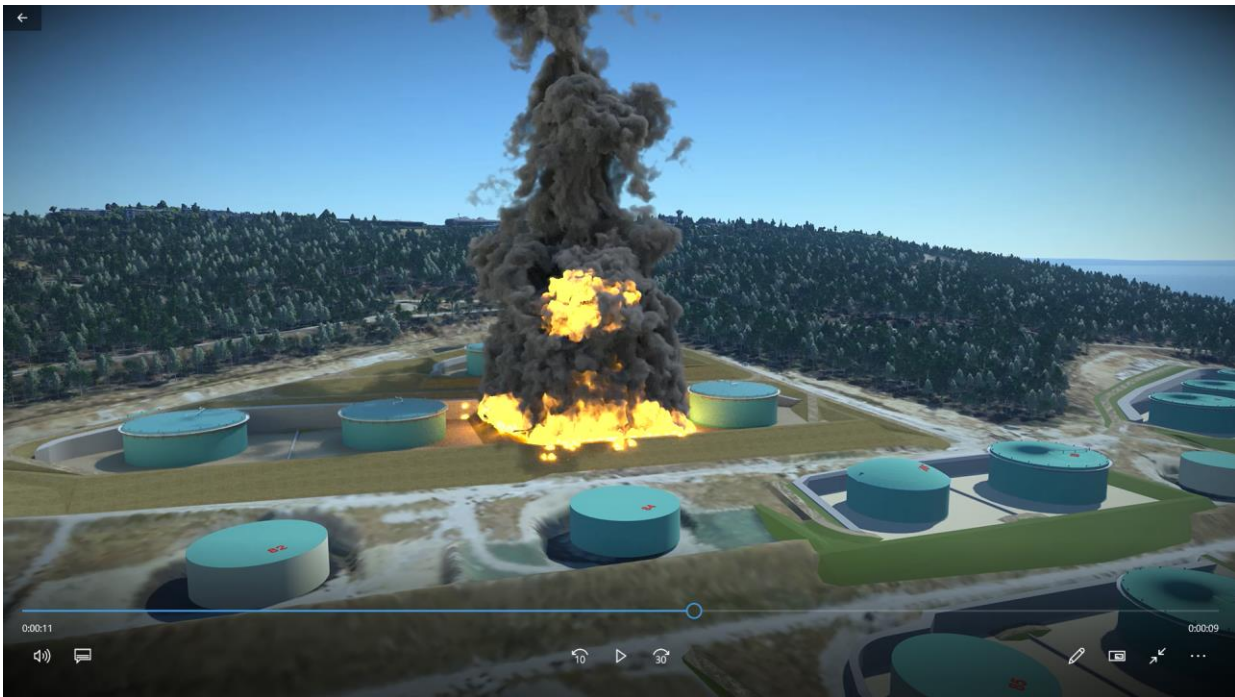
Above: A dike and full surface fire that if not extinguished could lead to a boilover.
