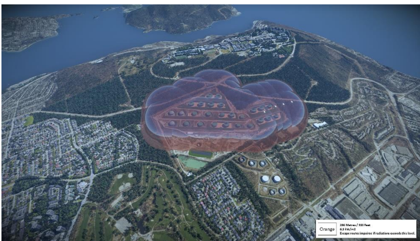
Burnaby Tank Farm and full surface fire heat map- Orange Zone.
