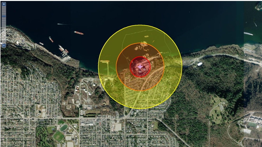
Figure 25: Radiation map for a BLEVE of the Propane vessel
