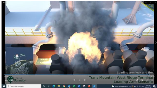
View #3 – View from tanker. Note that the view was adjusted in the dynamic model to view the leak / fire.
