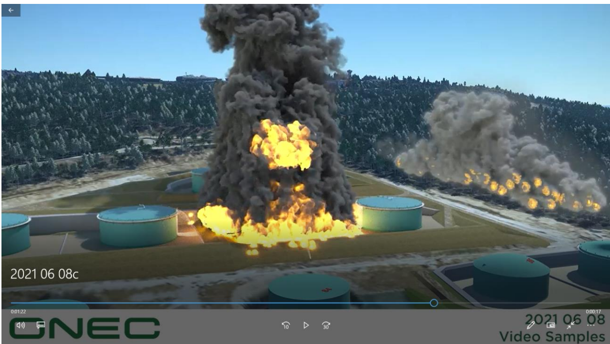
Full surface fire and dike fire or boilover that could lead to a wildfire in the surrounding treed areas. Note that multiple tanks in the vicinity are also at risk.
