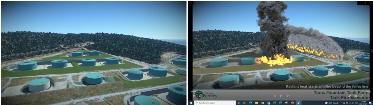
View #1- Overhead. The dynamic model view on right includes the tank and dike fire and the wildfire started from the radiant heat.
