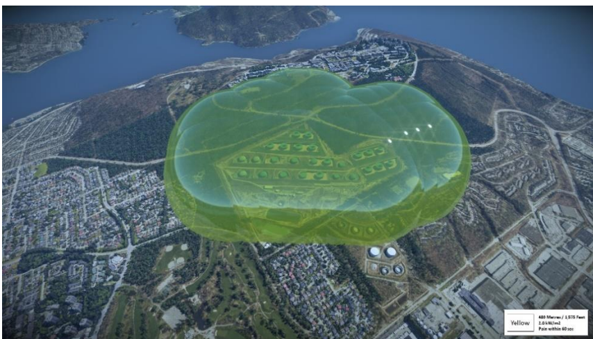
Burnaby Tank Farm and full surface fire heat map- Yellow Zone.
